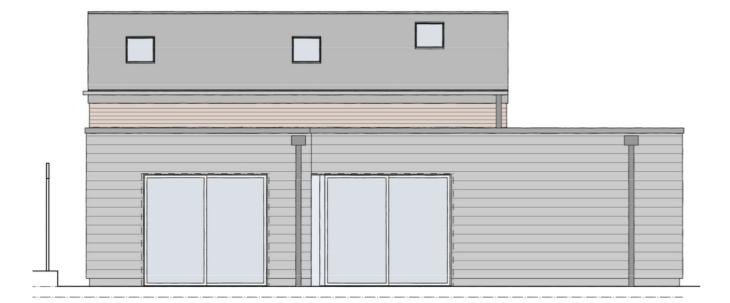
The building design is intended as a contemporary interpretation of the local building forms, with modern, robust materials such as fibre cement board cladding, London stock brickwork, slate and sedum roofs.
