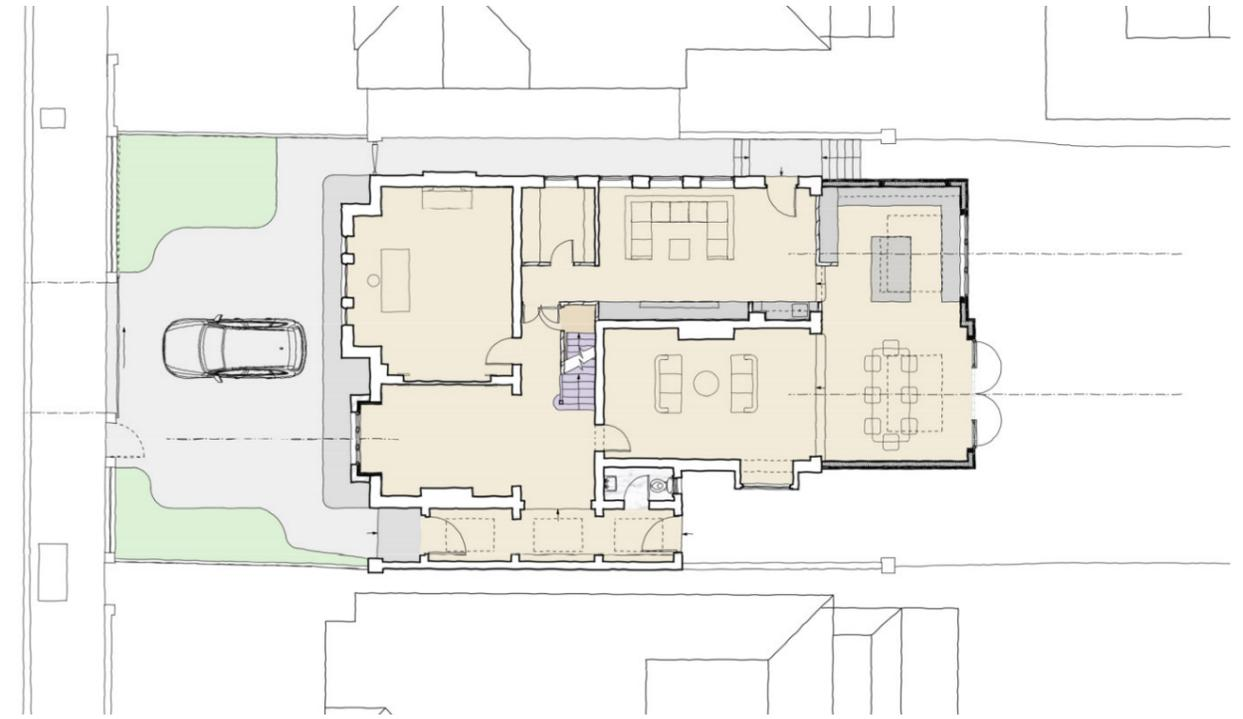
We formed a new front entrance porch, taking design cues from similar bays in the area. An unsympathetic non-original rear extension was removed and a large new rear extension inserted to provide a grand kitchen and dining area, with terraces above accessed from the rear bedrooms.
