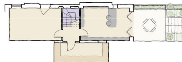
We removed the existing rear extension and replacing it with a contemporary pitched roof extension to create an open plan kitchen and dining area and improved access to the rear garden.
