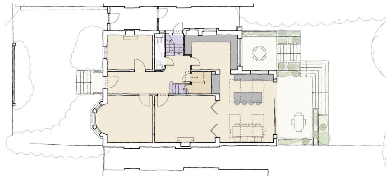
The bedroom spaces on the first floor were reorganised and a new staircase inserted up to the second floor. This, as well as the replacement of the small existing dormer with larger new zinc clad dormer allowed us to maximise the usable bedroom floor area on the top floor of the house.
