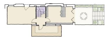
We removed the existing rear extension and replacing it with a contemporary pitched roof extension to create an open plan kitchen and dining area and improved access to the rear garden.
