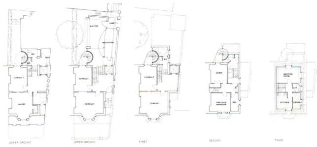
The existing building was sympathetically adapted to create additional accommodation for the medical centre. A sub-basement was excavated below the building to accommodate toilet facilities and a lift-pit, and a new 'bustle' constructed on the side elevation houses the lift shaft and landings essential for public access. The building makes a positive contribution to the streetscape with a new stained glass window, illuminated from within at night.
